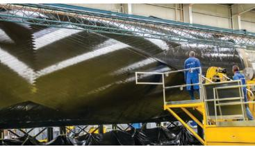
caused by friction at the rubber/mandrel interface. Orbital ATK's two-step alternative, made feasible by the large diameter of the case, improves consistency in the rubber layer's thickness. The rubber is then cured in the case in an autoclave at an unspecified temperature. Total postcured thickness of the case's carbon fiber wall is about 66 mm near the joints and approximately 25.4 mm in the cylinder region.
