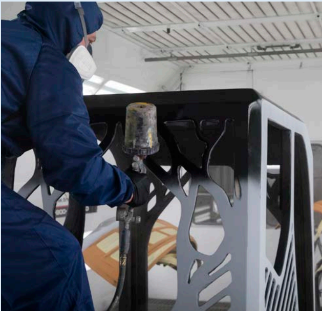
5 The proprietary primer coating facilitates easy application of paint (shown here) to the carbon-fiber/ABS cab.
