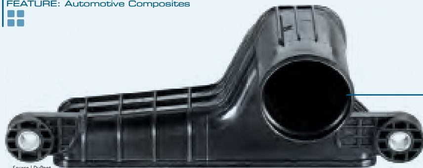
Tata Toya (Pune, India) manufactures three different charge air coolers installed on four different vehicles built by a major Indian automotive OEM. The coolers are made from a grade of DuPont Plastics' (Wilmington, Del.) 35-percent glass-filled Zytel PLUS and meet a continuous service requirement of 180°C/356°F. ■
