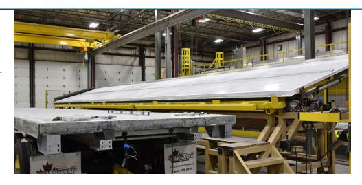
subsequently co-molded in a compression process to build the final MSC structures, which form the walls and floors of a *Cold Chain* truck.
